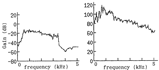
Fig.2 Experiment result when the noise is male voice with percussion. (a) Transfer function of adaptive filter. (b) spectrum of noise.
