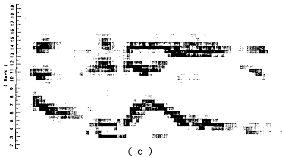
Fig.3 Formant extraction for open word male spoke (a) DFT spectrogram (b) output of proposed auditory model (c) output of the formant extraction NN
