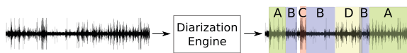
Figure 1: Overview of speaker diarization. From an input audio signal, segment the signal into nonspeech and speech segments, the latter labeled by speaker (e.g., A, B, C, D).
