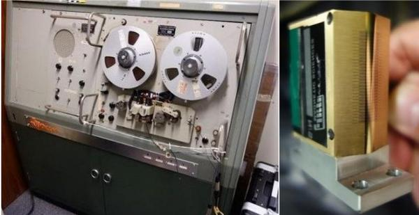
Figure 1: (left): The SoundScriber device used to decode 30 track analog tapes, and (right): The UTD-CRSS designed read-head decoder retrofitted to the SoundScriber [13]
