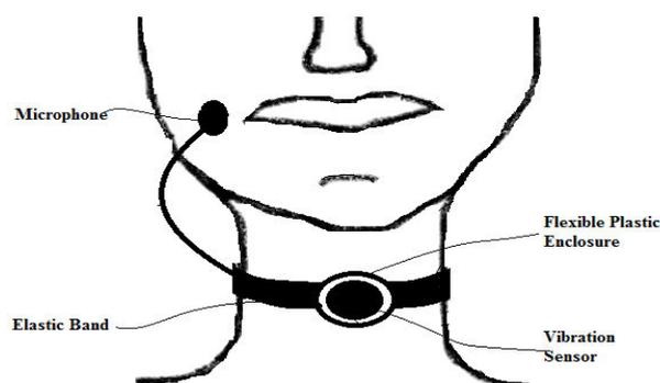
Figure 3: Placement of the sensor and microphone.
