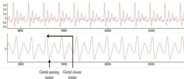
Figure 2: Screenshot of the interface showing the speech waveform on the top panel and the glottal instants on the bottom panel.
