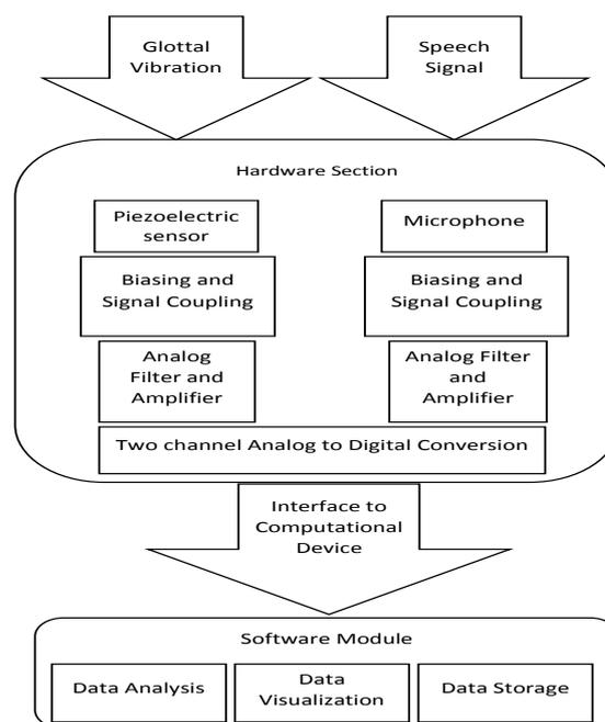
Figure 1: Block diagram representation of the system.
