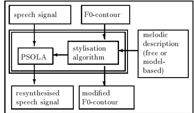
Figure 2 shows the main components of the labelling and test environment (surrounded by double lines) and its input and output files.
