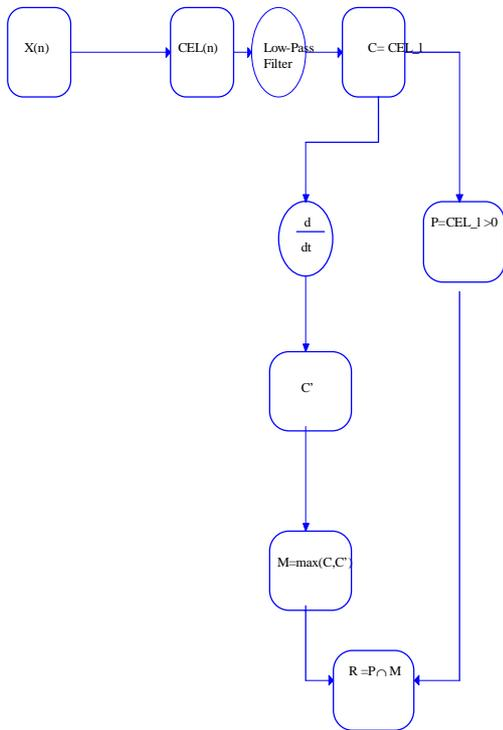
figure 1 : Rupture detection algorithm using LEC function.
