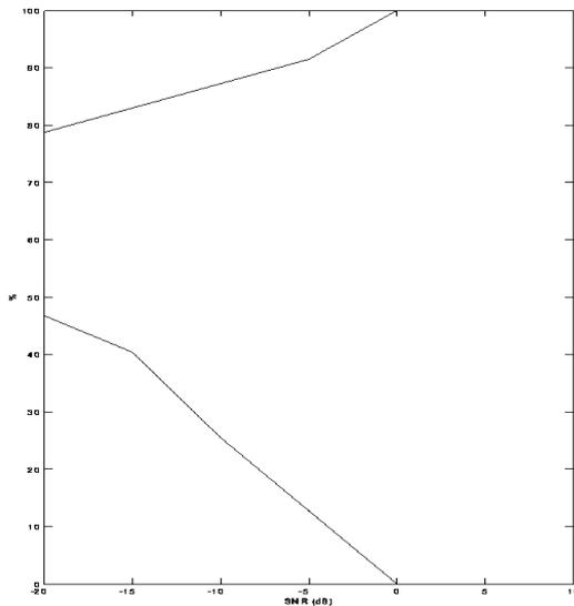
figure 5 : Correct detection rate (upper curve) and False alarm detection rate ( lower curve), relative to SNR with  $\lambda=0.5$ .
